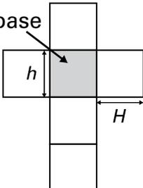
$$\begin{aligned} V &= A_{\text{base}} \times H \\ &= A_{\text{carré}} \times H \\ &= b \times h \times H \end{aligned}$$
