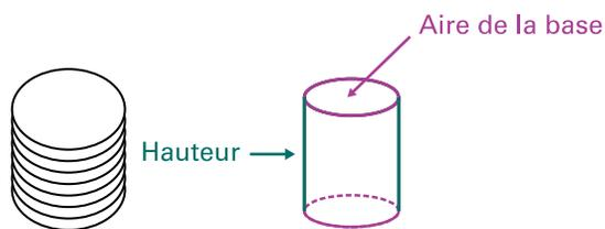
$$\begin{aligned}V_{cylindre} &= A_{base} \times H \\ &= A_{disque} \times H \\ &= \pi \times r^2 \times H\end{aligned}$$
