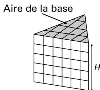
$$\begin{aligned}V &= A_{base} \times H \\ &= A_{triangle} \times H \\ &= \frac{b \times h}{2} \times H\end{aligned}$$
