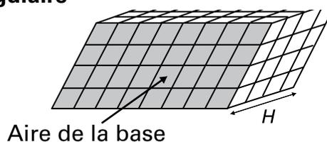
$$\begin{aligned}V &= A_{base} \times H \\ &= A_{parallélogramme} \times H \\ &= b \times h \times H\end{aligned}$$
